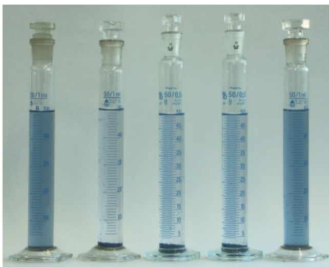
Figure 1 Flocculation of the dye solution (80 mg/L) after adding different quantities of TP1 (without centrifugation); 1–0.3 mL = 187.5 mg/g dye; 2–0.6 mL = 375 mg/g; 3–0.7 mL = 437.5 mg/g; 4–0.8 mL = 500 mg/g; and 5–1.0 mL = 625 mg/g. [Color figure can be viewed in the online issue, which is available at www.interscience.wiley.com .]
